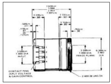
Sciencetech offers intensifier systems for photodiode array detector cameras and CCD cameras. The system could be an add-on to Sciencetech multichannel detectors or a retrofit to other CCD cameras. This add-on is for nongating applications. A Generation II Multichannel plate image intensifier(inverter tube) is optically coupled to the active detector with a high-throughput, multi-element lens system.
