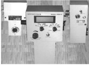
The Sciencetech PMH-02 Photomultiplier housing is a self-contained compact unit for operation of photomultipliers in analog mode. The PMH-02 housing operates at room temperature. The PMH-04 is a Peltier cooled unit (see corresponding brochure).
