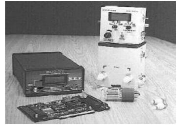
Cooling a photomultiplier tube helps substantially in the detection of weak signals. The dark current which sets the low detection limit is reduced by cooling the photocathode. Sciencetech Cooled Photomultiplier systems include a PMH-04 photomultiplier housing with thermoelectric cooling and a temperature controller.
