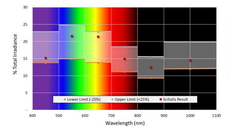
15.1774% 400-500 Class A nm = 500-600 21.5593% Class A nm = 600-700 21.3764% Class A nm = Class A 700-800 nm = 14.9445% 800-900 nm = 12.4609% Class A 900-1100 nm = 14.4815% Class A
