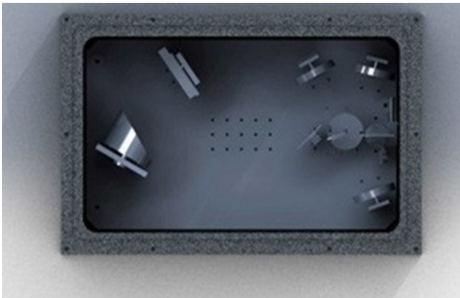
Optical Layout for SPS300 Sample Chamber
